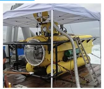
This highly maneuverable craft is powered entirely by Lithium batteries housed in external pods. The submarine accommodates two passengers and a pilot and uses a main propulsion motor and four thrusters for excellent maneuvering capability. It is equipped with powerful LED underwater lights to enhance viewing in deep/dark water or to bring out the natural colors not seen with ambient light at depth.
